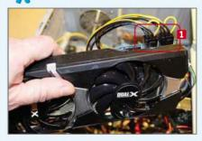
Most modern graphics cards are quite big, so make sure you have plenty of room inside your PC's case. This might mean you have to temporarily disconnect some cables and possibly relocate your hard drives. The first and most important thing to do is to connect power to the card, using the supplied Molex-to-six-pin adapters. 🚹
