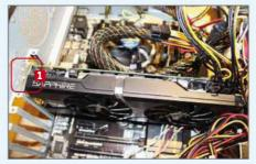
Insert the card into a spare PCI-Express slot and push down hard so the locking clip pops into place, securing the card into position. Screw the card into the chassis 11 to prevent movement, then connect your monitors. This card comes with outputs for DVI, HDMI, DisplayPort and VGA.
